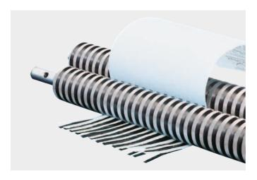
**SOLID STEEL CUTTING SHAFTS** Robust and durable: high-quality paper clip proof cutting shafts from special hardened steel. Lifetime guarantee on the solid steel cutting shafts under conditions of fair wear and tear.
